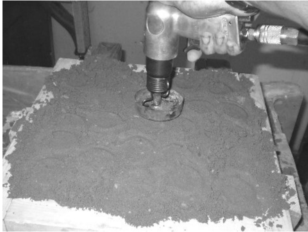
Figure III-14: Finishing the ramming
