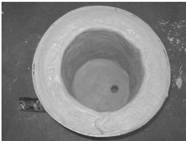
Figure VI-7: Furnace ready to dry
